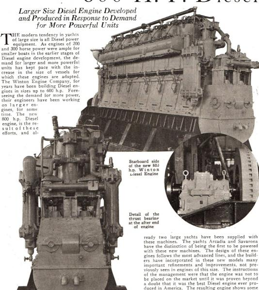
Forward end of machine showing its compact and close arrangement
