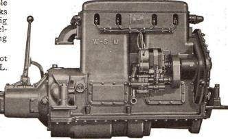
HIGH SPEED 48 to 60 H. P. 1,000 to 1,400 R.P.M. Weight 1,250 lbs MEDIUM DUTY 28 to 45 H. P. 600 to 900 R. P. M. Weight, 1,450 lbs.
