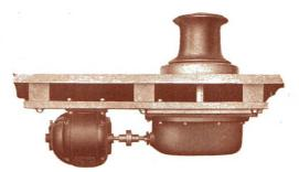
A-E-CO Electric Windlass, Gypsey Type for rope or cable, handles anchor, sail, small boats or warping lines—compact, powerful, economical. Occupies very little space above or below deck—easy to install—easy to operate. You just step on the button and the windlass does the rest. Takes very little power. A handsome machine with polished bronze head and mahogany base. Also furnished in wildcat type for chain. The most popular windlass on the market. Installed on hundreds of yachts and powerboats.
