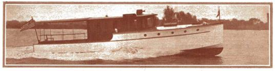
Nomabin—a 44 ft. day cruiser designed by Hacker & Fermann and built by Defoe—equipped with one 6 cyl. 200 h.p. Hall Scott Marine motor giving speed of 20 miles per hour.
