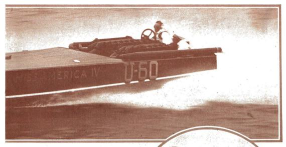
motors placed well aft in the hull. The shape of the underbody was slightly different, yet in all other ways the hulls and power plans were identical. Hyde wheels were used, Miss America III using one 20 x 40, Miss America IV, 21 x 38 and Miss America V, 21 x 37. Delco starting and ignition was used in all the boats.
