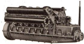
MODEL IM-1242—12 cylinder Sweepstakes Type. Designed originally for the Sweepstakes Race and winner of both the 1926 and 1925 Sweepstakes. Develops 500 H. P. at 2500 R. P. M. Weight 1140 lbs. Speed up to 67 miles per hour. Price, complete with equipment, \$12,000.00.
