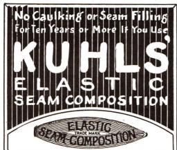
K UHLS' Elastic Seam Composition is the most satisfactory and durable filler you can use for deck seams and Kuhls' Elastic Glazing Composition for top, sides and bottom seams. One filling lasts for years. It sets semi-hard, but never gets brittle, adhering tightly to the sides of the seams, and retains all its original elasticity through many years of hard service.
