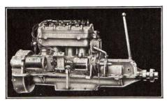
BRENNAN Model E-4 Medium Duty, 35 H.P. at 1000 R.P.M. High Speed, 50 H.P. at 1600 R. P. M. Bore 4½". Stroke 5".
